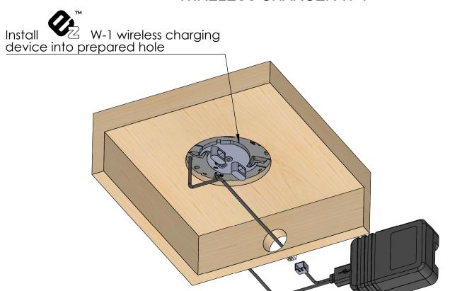
If wireless charger device fits properly to the hole and you feel that device can not be pushed deeper please twist this part in CW direction to lock
